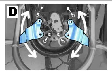
\* The original brackets indicated in blue can be rotated. Remove the 4 screws of the rear fender in E, then loosen the screws in F. Fit the Unit garage frame in point B2, and retighten the screws F, and refit the rear fender.
