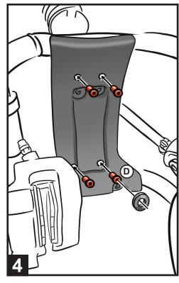
**EN**\_Remove the seat, the original mudguard and the rear wheel.
