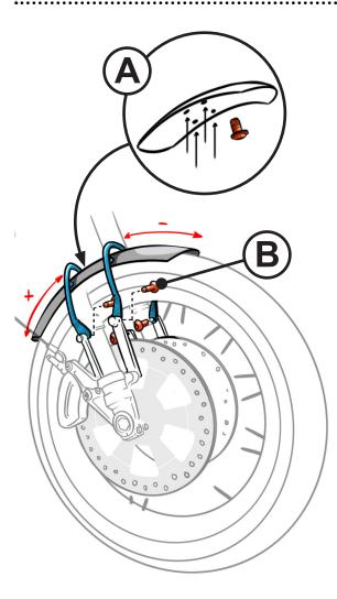
**EN** Mount the mudguard on the arched frames using the M6 screws (A) from below. As indicated in the drawing, we recommend turning the longer part of the mudguard towards the engine.
