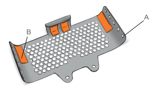
**EN** Attach the 4 included pieces of foam tape as shown in the image above. Mount the radiator protection using the 2 original screws at the top of the radiator.
