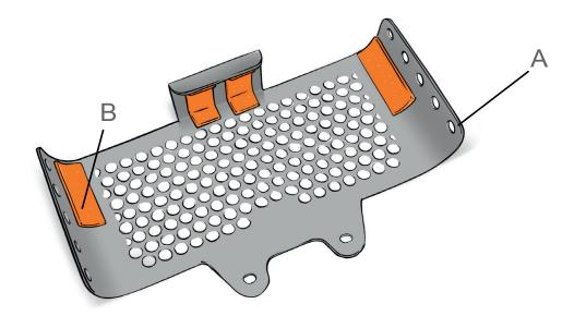
**EN** Attach the 4 included pieces of foam tape as shown in the image above. Mount the radiator protection using the 2 original screws at the top of the radiator.
