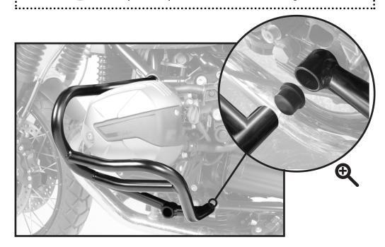
EN For mounting the crash bars code 1625 and 1691 on Euro 5 models, it's necessary to add the spacer supplied in the kit as indicated: the spacer it's needed only on the left side of the bike!
