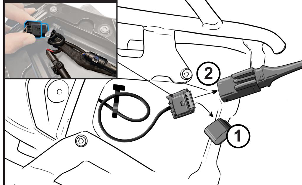
**EN** To connect the rear light, use the plug indicated in the figure (after removing the protective cap): it is located in the compartment under the seat in the rear area of the motorbike.
