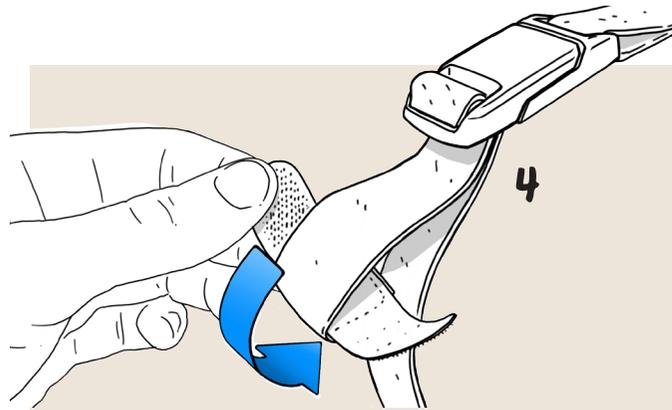
4\_ On each end of a buckle open the velcro strips, and roll up the strap.
