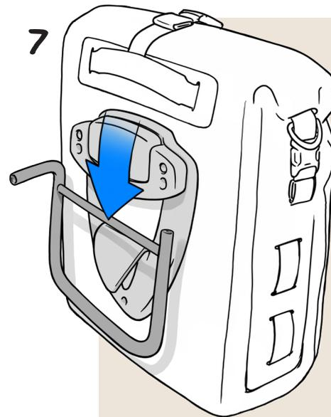
7\_ the back of the pannier is fitted with a quick-lock mechanism. Slide it onto the Unitgarage subframe mounted to your motorcycle.
