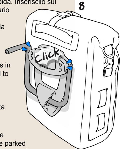
8\_ Push down until the mechanism clicks in place. The bag is now securely fastened to your motorcycle.
